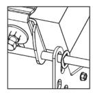
3. Slide the hinge axle rod through both upper hinge leaves.
