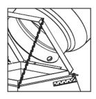
4. Slide lower hinge leaves onto axle rod and up to curb surface that works best for the installation. Using the supplied self tapping screws connect it to the curb.
