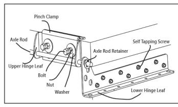
1. Loosely assemble upper hinge leaf as shown. The oval holes on the pinch clamp over lay the threaded holes of the upper hinge. Assemble bolt, nut, washer and thread into the upper leaf.
