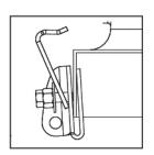
6. Slide the axle rod retainer onto the axle rod on both sides
