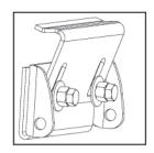
5. Return to upper hinge leaves and tighten the bolt and the lock nut to secure the assembly. Don't over tighten bolts. You want them to firmly contact the lid but not open the J-hook.
