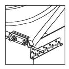
8. If the stainless steel axle rod extends more than 2" past the lower hinge leaf, it must be cut offusing a powered abrasive wheel.
