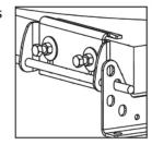
2. Slide upper hinge leaf on lid base. Squeeze pinch clamp down and upper hinge leaf up so they are tight. Hand tighten bolts to temporary hold upper hinge leaf in place. This aids in axle rod alignment in step 3.
