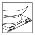
7. Screw chains to front corner of curb. Lean fan back to adjust chain length. Fan should be open so gravity pulls if back against chains. Screw chain into fan base.
