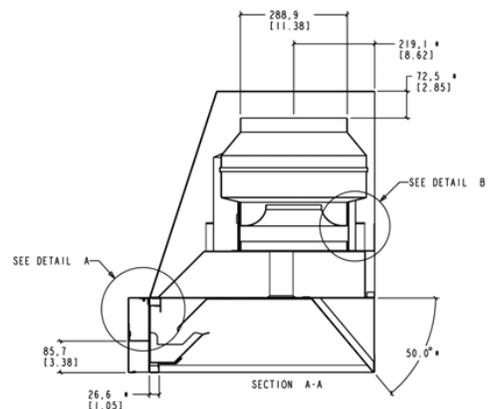
\* The assembly must be clear of combustible materials and semi-combustible according to the Building Code
