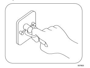
Once the fire suppression system is actuated, equipment to shut off the fuel supply to the cooking appliances will operate. ► 3. Call the local fire department or emergency number.
