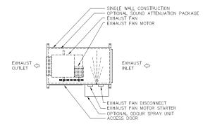
The UL/ULC listing allows recirculation only with electric cooking and only up to 80% of the total exhausts air.
