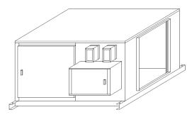
The unit casing is 16-gauge steel, primed and painted suitably reinforced to ensure rigidity. An optional sound attenuation package is available for the interior of the fan unit. This sound package is highly recommended on all indoor units. The KESF unit is supported by channels running along the length of each side. Lifting and support points are at the four corners of the KESF unit, at the ends of these channels. An access door is provided to the exhaust fan motor and drives section.
