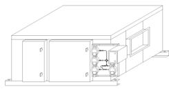
Pressure tubing from the pressure switches is run inside along the top of the unit to pressure probes located in front and behind each filter section. The Firestat is located at the exhaust inlet end and mounted on the same side as the CC20 panel.
