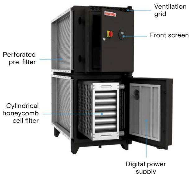
As the air passes through the combined ionizer/collector cell, the grease particles in the air stream are negatively charged with a flood of electrons that are produced during the charging process. The negatively ionized particles are attracted by the grounded collectors in the diffusion process. Therefore, they settle out of the air flow and stick to the sides of the cylinders that are in the cylindrical honeycomb cell filter.
